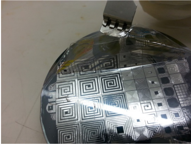
Scalable manufacture using microfabrication techniques for silicon wafer processing
